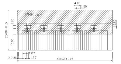
NOTE) \*1 The shaded area shows the solder resist treatment.
