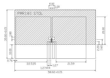
NOTE) \*1 The shaded area shows the solder resist treatment.
