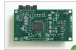
Motor Control Evaluation System
