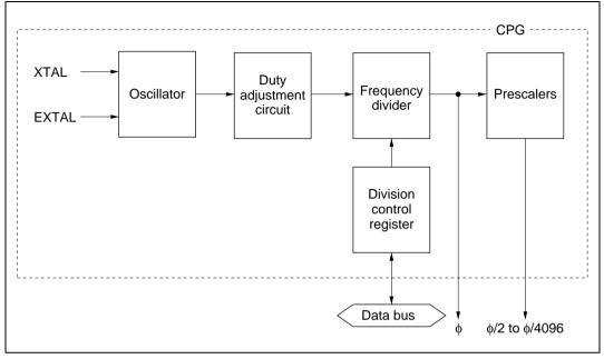
Figure 20.1 Block Diagram of Clock Pulse Generator
