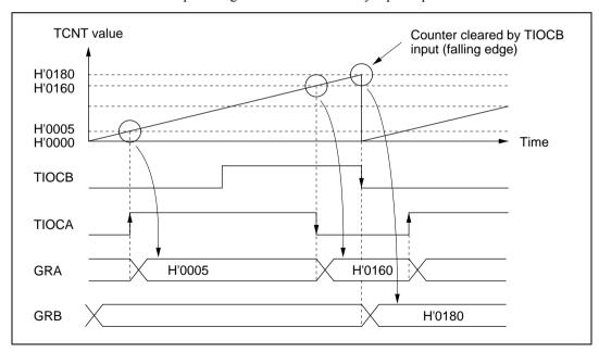
Figure 10.24 Input Capture (Example)
