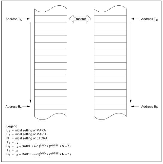
Figure 8.8 Operation in Normal Mode
