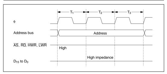
Figure 2.18 Pin States during Access to On-Chip Supporting Modules
