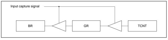
Figure 10.47 Input Capture Buffering
