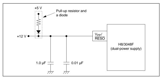
Figure 19.25 V<sub>PP</sub> Power Supply Circuit Design (Example)
