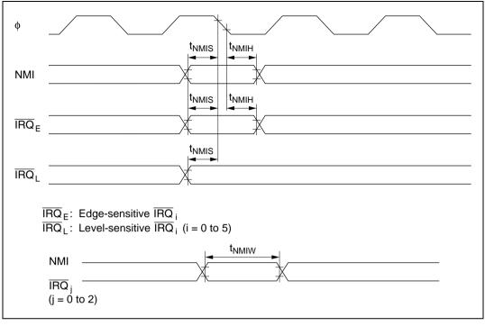
Figure 22.20 Interrupt Input Timing
