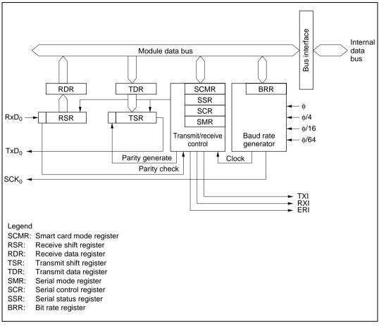
Figure 14.1 Smart Card Interface Block Diagram
