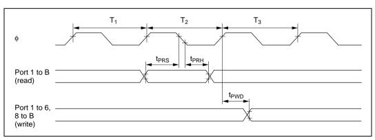
Figure 22.23 TPC and I/O Port Input/Output Timing
