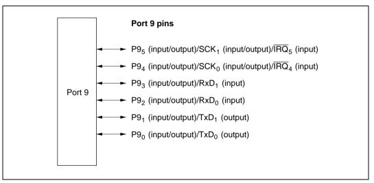
Figure 9.9 Port 9 Pin Configuration
