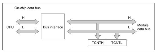
Figure 10.6 Access to Timer Counter (CPU Writes to TCNT, Word)
