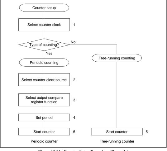
Figure 10.14 Counter Setup Procedure (Example)
