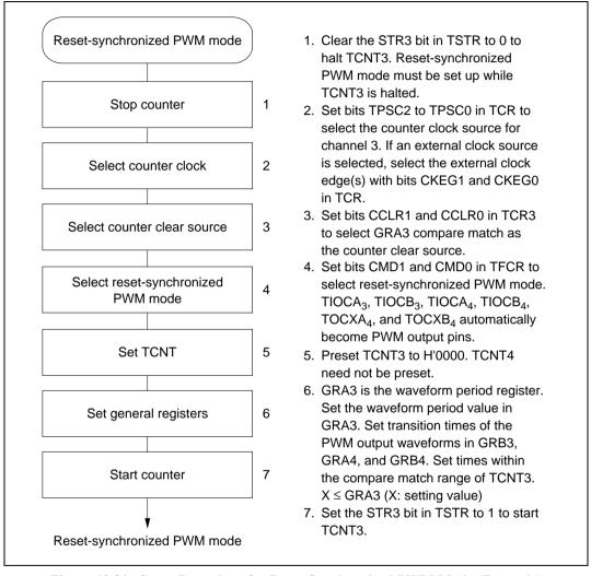
Figure 10.31 Setup Procedure for Reset-Synchronized PWM Mode (Example)
