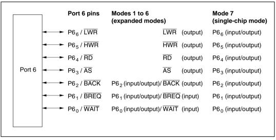
Figure 9.6 Port 6 Pin Configuration
