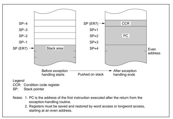
Figure 2.14 Stack Structure after Exception Handling
