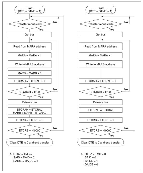
Figure 8.11 Block Transfer Mode Flowcharts (Examples)
