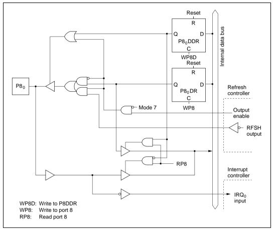
Figure C.8 (a) Port 8 Block Diagram (Pin P8<sub>0</sub>)
