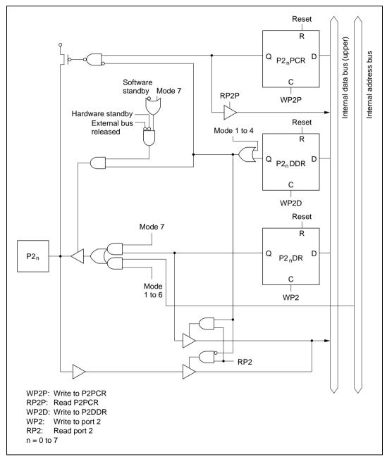
Figure C.2 Port 2 Block Diagram
