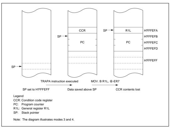
Figure 4.7 Operation when SP Value is Odd
