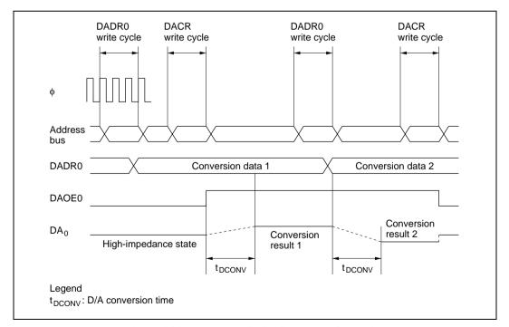
Figure 16.2 Example of D/A Converter Operation
