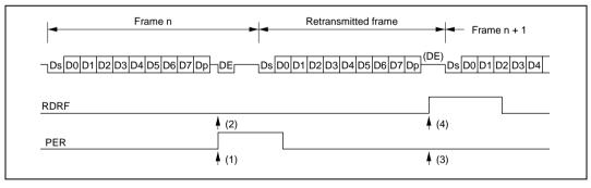
Figure 14.11 Retransmission in SCI Receive Mode
