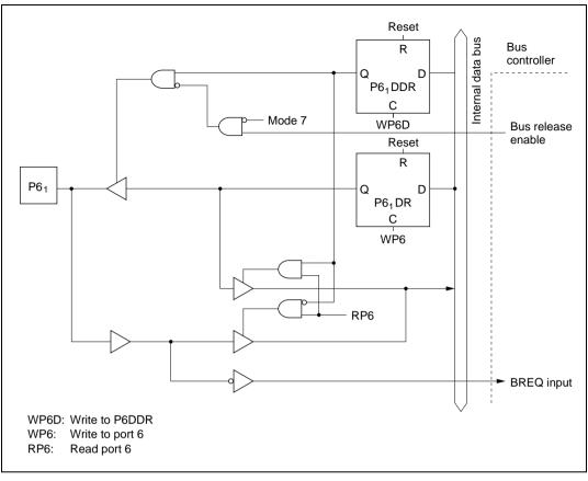
Figure C.6 (b) Port 6 Block Diagram (Pin P6<sub>1</sub>)
