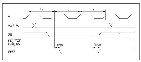
Figure 22.17 PSRAM Bus Timing (Refresh Cycle): Three-State Access
