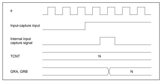
Figure 10.25 Input Capture Signal Timing
