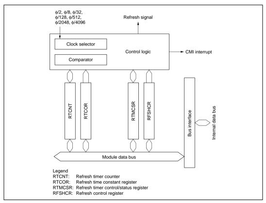
Figure 7.1 Block Diagram of Refresh Controller
