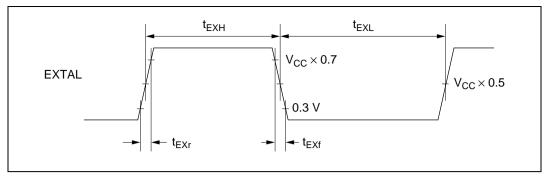
Figure 20.6 External Clock Input Timing
