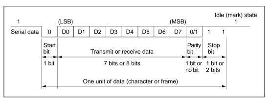
Figure 13.2 Data Format in Asynchronous Communication (Example: 8-Bit Data with Parity and 2 Stop Bits)
