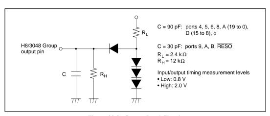
Figure 22.3 Output Load Circuit
