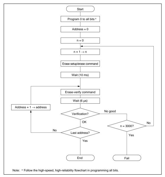
Figure 19.18 High-Speed, High-Reliability Erasing
