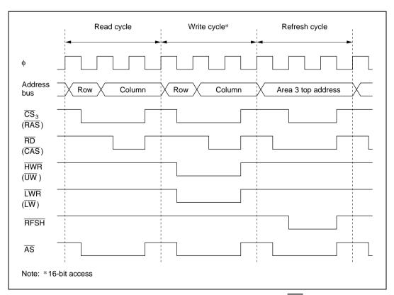
Figure 7.5(1) DRAM Control Signal Output Timing (2WE Mode)
