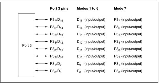
Figure 9.3 Port 3 Pin Configuration
