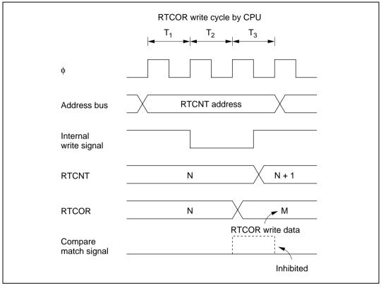
Figure 7.22 Contention between RTCOR Write and Compare Match
