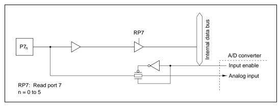
Figure C.7 (a) Port 7 Block Diagram (Pins P7<sub>0</sub> to P7<sub>5</sub>)
