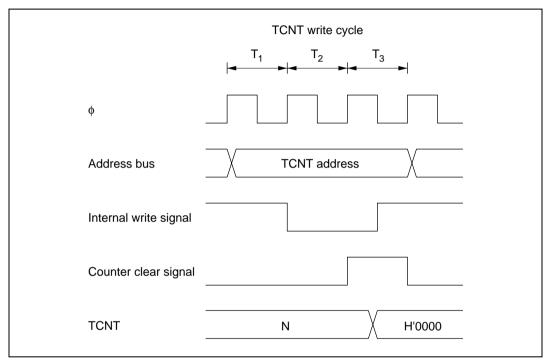
Figure 10.61 Contention between TCNT Write and Clear
