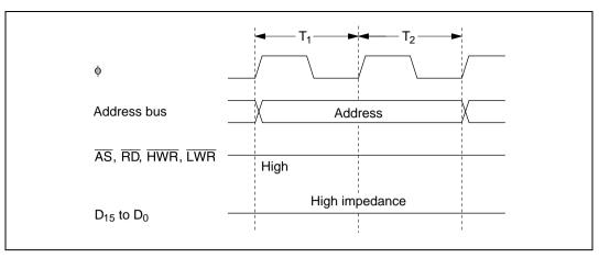
Figure 2.16 Pin States during On-Chip Memory Access
