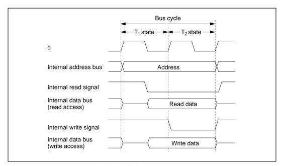
Figure 2.15 On-Chip Memory Access Cycle
