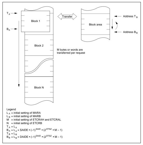
Figure 8.10 Operation in Block Transfer Mode
