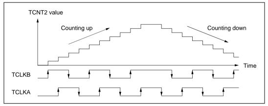
Figure 10.44 Operation in Phase Counting Mode (Example)
