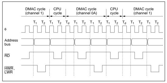
Figure 8.19 Timing of Multiple-Channel Operations
