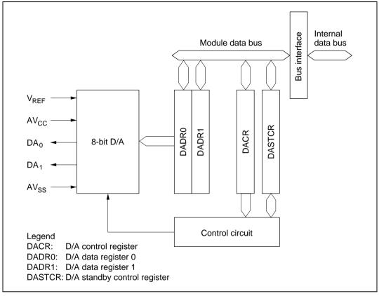
Figure 16.1 D/A Converter Block Diagram
