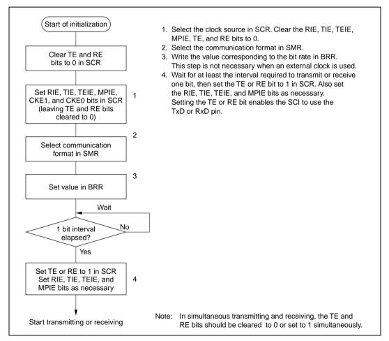
Figure 13.15 Sample Flowchart for SCI Initialization
