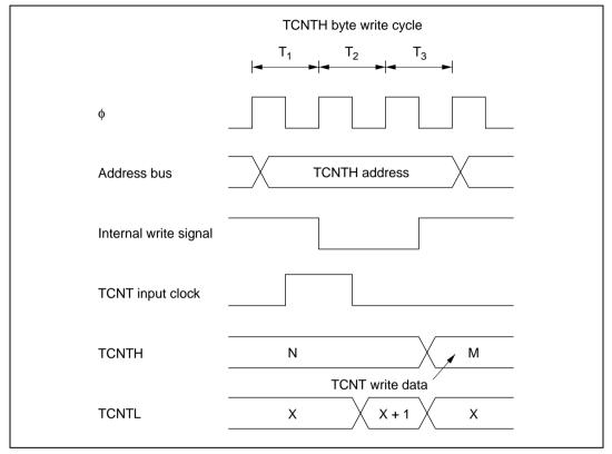
Figure 10.63 Contention between TCNT Byte Write and Increment
