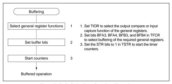
Figure 10.48 Buffering Setup Procedure (Example)
