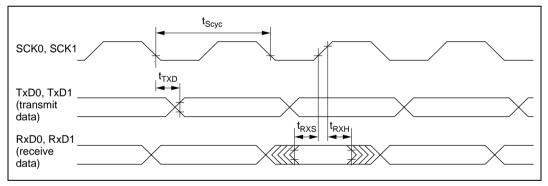
Figure 22.27 SCI Input/Output Timing in Synchronous Mode
