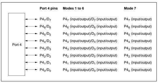
Figure 9.4 Port 4 Pin Configuration
