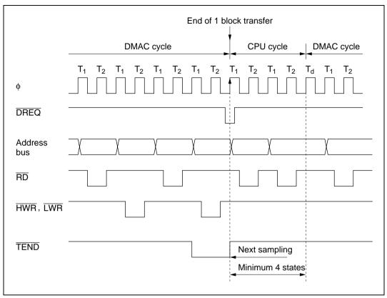
Figure 8.18 Timing of DMAC Activation by Falling Edge of DREQ in Block Transfer Mode
