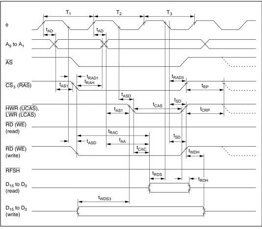
Figure 22.13 DRAM Bus Timing (Read/Write): Three-State Access
