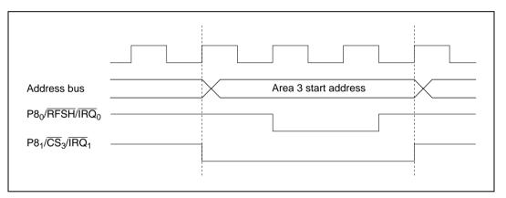
Figure 7.23 Operation when DRAM/PSRAM Connection is Switched
