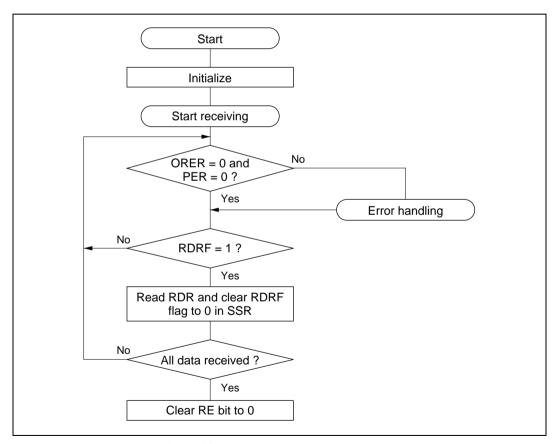
Figure 14.7 Receive Flowchart (Example)
