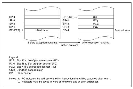
Figure 4.6 Stack after Completion of Exception Handling
