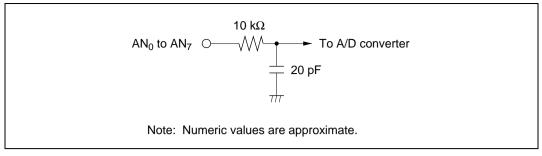
Figure 15.8 Analog Input Pin Equivalent Circuit
