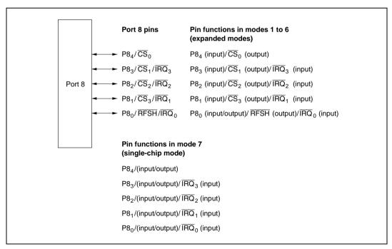
Figure 9.8 Port 8 Pin Configuration
