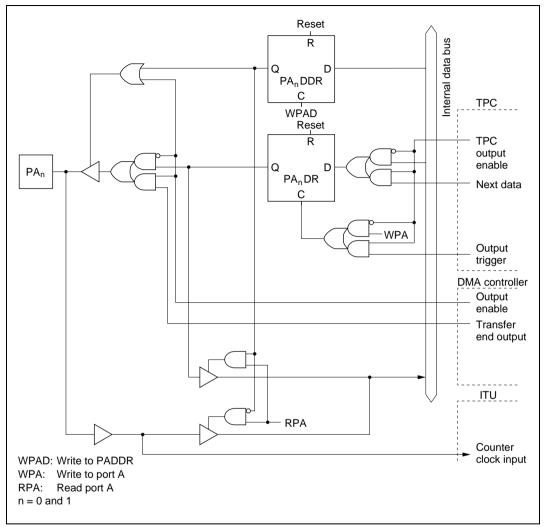
Figure C.10 (a) Port A Block Diagram (Pins PA<sub>0</sub> and PA<sub>1</sub>)
