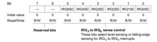
ISCR is initialized to H'00 by a reset and in hardware standby mode.
