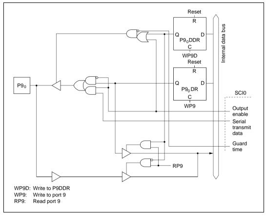
Figure C.9 (a) Port 9 Block Diagram (Pin  $P9_0$ )
