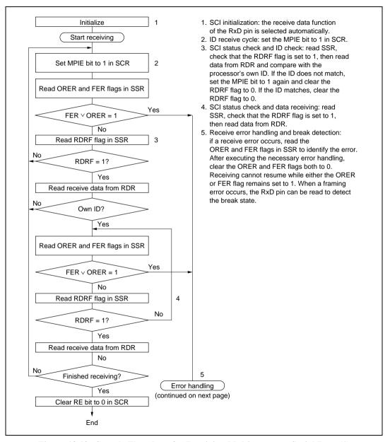
Figure 13.12 Sample Flowchart for Receiving Multiprocessor Serial Data (1)
