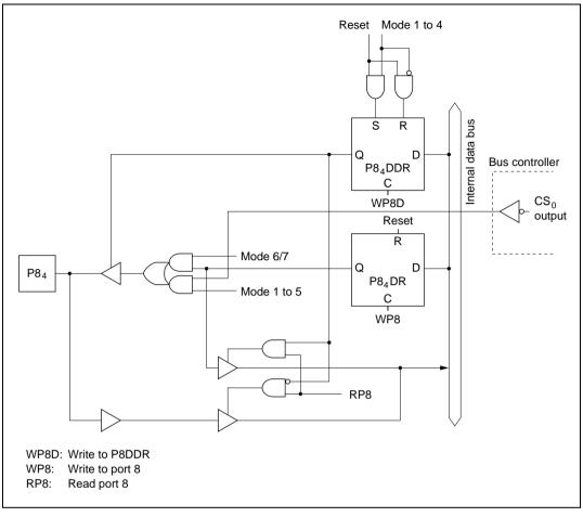
Figure C.8 (c) Port 8 Block Diagram (Pin P84)
