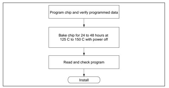
Figure 18.6 Recommended Screening Procedure
