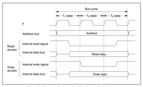
Figure 2.17 Access Cycle for On-Chip Supporting Modules
