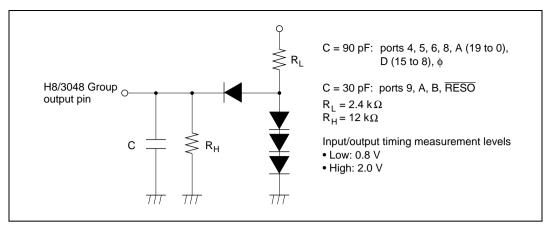
Figure 22.6 Output Load Circuit
