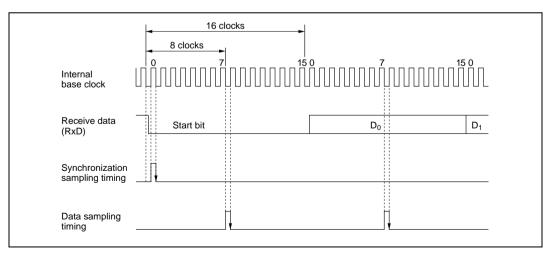
Figure 13.21 Receive Data Sampling Timing in Asynchronous Mode
