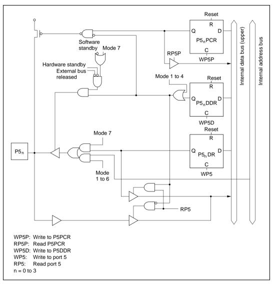
Figure C.5 Port 5 Block Diagram
