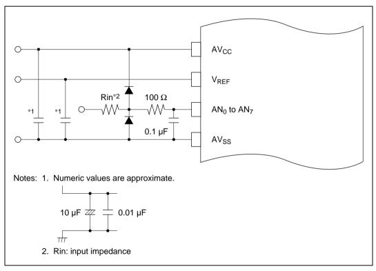
Figure 15.7 Example of Analog Input Protection Circuit
