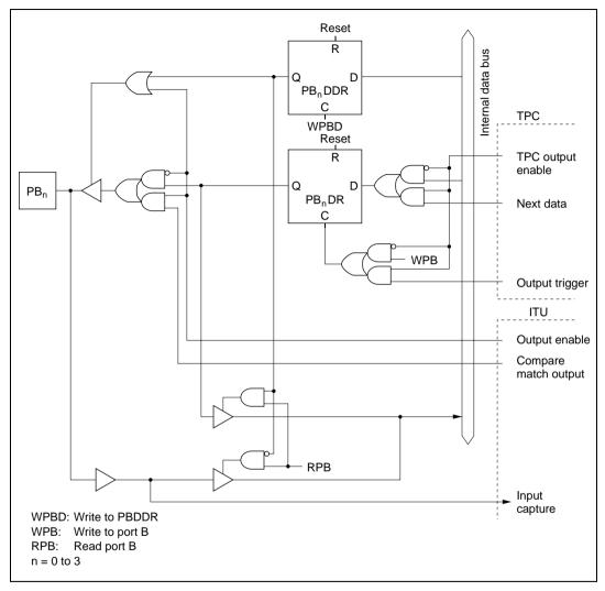
Figure C.11 (a) Port B Block Diagram (Pins PB<sub>0</sub> to PB<sub>3</sub>)
