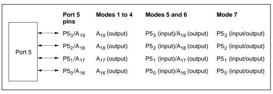
Figure 9.5 Port 5 Pin Configuration
