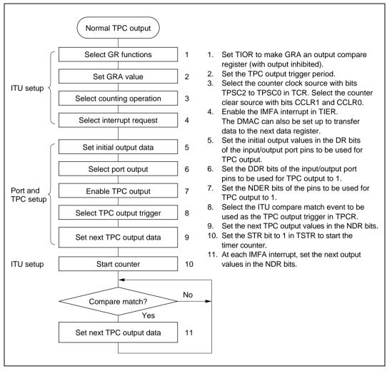
Figure 11.4 Setup Procedure for Normal TPC Output (Example)
