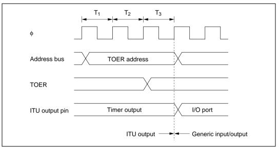
Figure 10.54 Timing of Disabling of ITU Output by Writing to TOER (Example)
