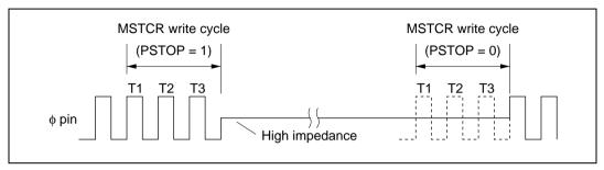
Figure 21.3 Starting and Stopping of System Clock Output
