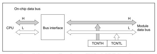
Figure 10.10 Access to Timer Counter (CPU Reads TCNT, Upper Byte)
