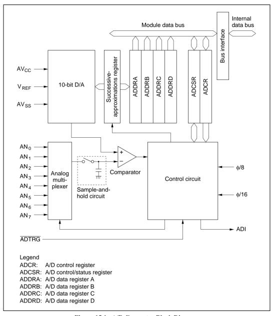
Figure 15.1 A/D Converter Block Diagram
