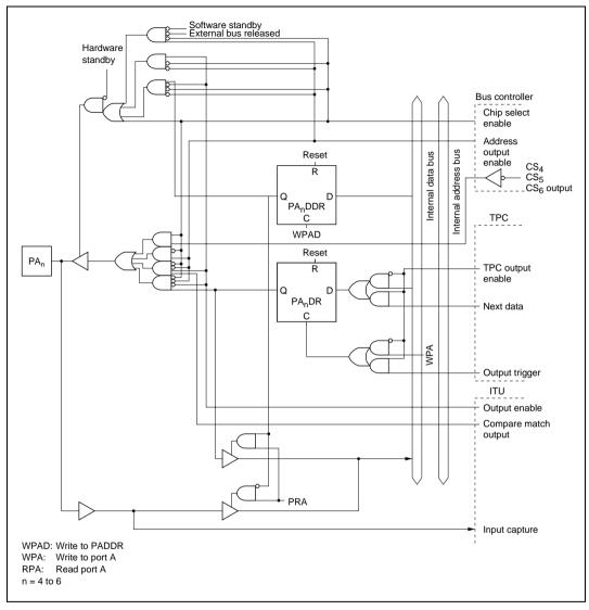
Figure C.10 (c) Port A Block Diagram (Pins PA<sub>4</sub> to PA<sub>6</sub>)
