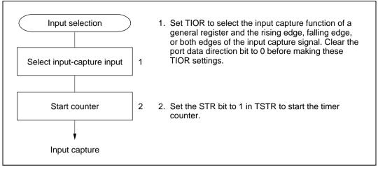
Figure 10.23 Setup Procedure for Input Capture (Example)
