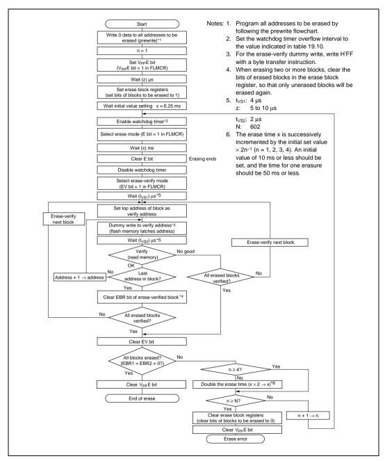
Figure 19.12 Multiple-Block Erase Flowchart
