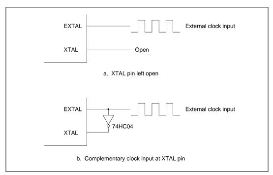
Figure 20.5 External Clock Input (Examples)
