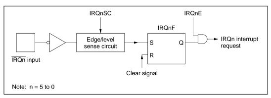
Figure 5.2 Block Diagram of Interrupts IRQ<sub>0</sub> to IRQ<sub>5</sub>
