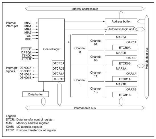
Figure 8.1 Block Diagram of DMAC
