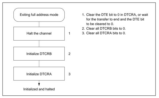
Figure 8.23 Procedure for Exiting Full Address Mode (Example)
