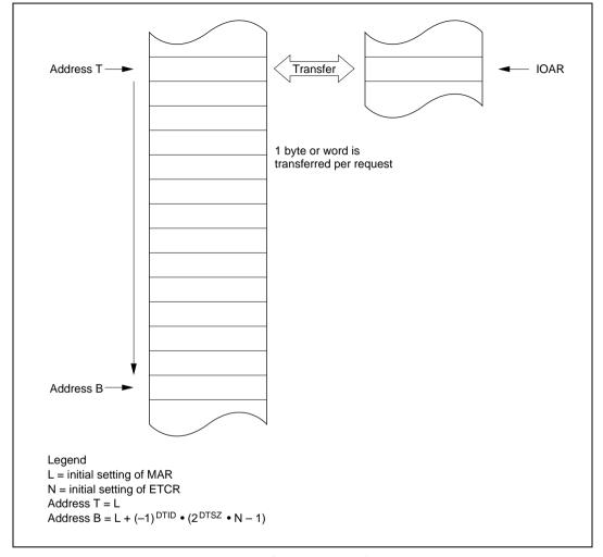
Figure 8.2 Operation in I/O Mode
