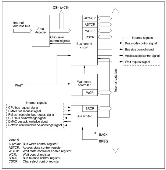
Figure 6.1 Block Diagram of Bus Controller
