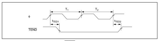
Figure 22.28 DMAC TEND Output Timing for 2 State Access
