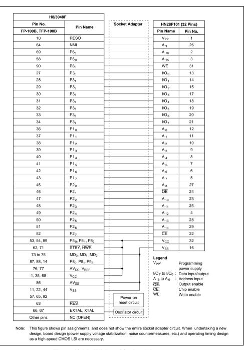
Figure 19.16 Wiring of Socket Adapter
