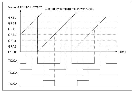
Figure 10.27 Synchronization (Example)
