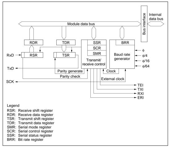
Figure 13.1 SCI Block Diagram
