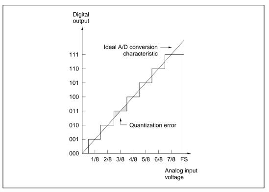
Figure 15.9 A/D Converter Accuracy Definitions (1)
