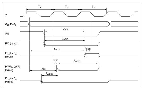
Figure 22.8 Basic Bus Cycle: Three-State Access
