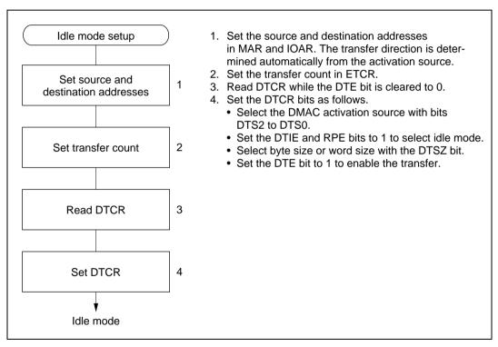
Figure 8.5 Idle Mode Setup Procedure (Example)
