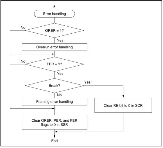
Figure 13.12 Sample Flowchart for Receiving Multiprocessor Serial Data (2)
