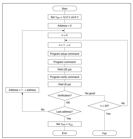
Figure 19.17 High-Speed, High-Reliability Programming
