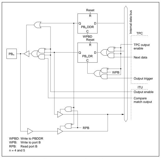
Figure C.11 (b) Port B Block Diagram (Pins PB<sub>4</sub> and PB<sub>5</sub>)
