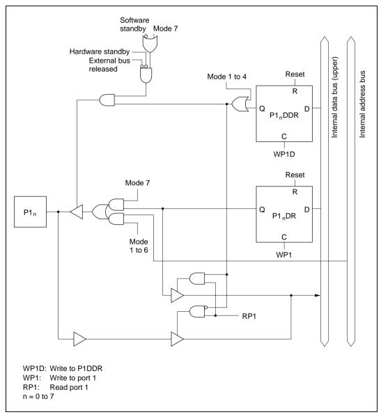
Figure C.1 Port 1 Block Diagram
