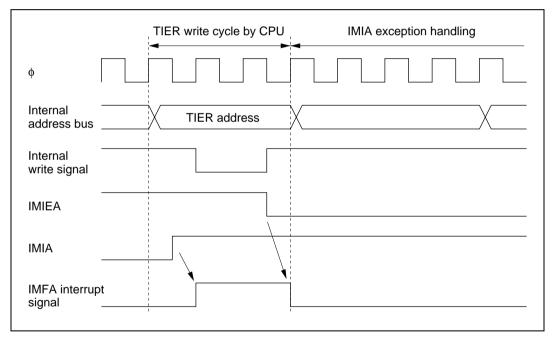
Figure 5.8 Contention between Interrupt and Interrupt-Disabling Instruction
