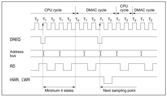
Figure 8.16 Timing of DMAC Activation by Falling Edge of DREQ in Normal Mode
