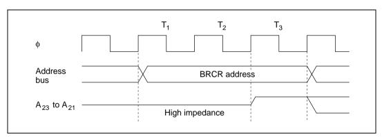
Figure 6.22 BRCR Write Timing
