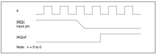
Figure 5.3 Timing of Setting of IRQnF
