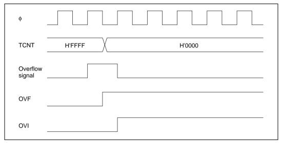
Figure 10.59 Timing of Setting of OVF
