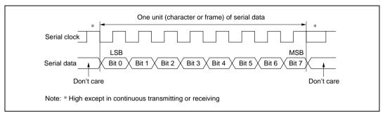
Figure 13.14 Data Format in Synchronous Communication
