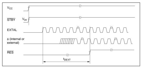
Figure 20.7 External Clock Output Settling Delay Timing
