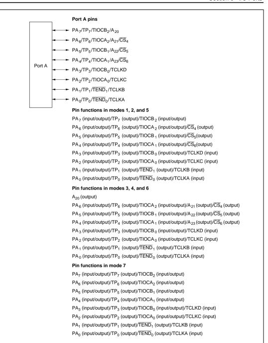
Figure 9.10 Port A Pin Configuration
