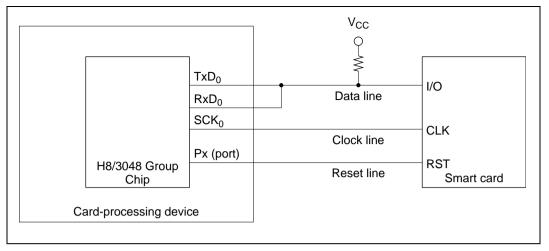
Figure 14.2 Smart Card Interface Connection Diagram
