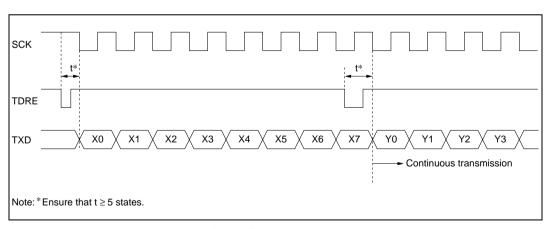
Figure 13.22 Serial Clock Transmission (Example)
