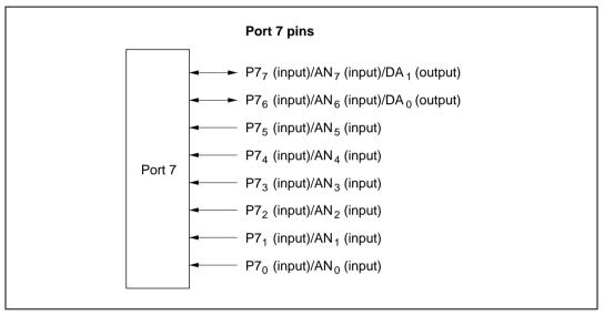
Figure 9.7 Port 7 Pin Configuration
