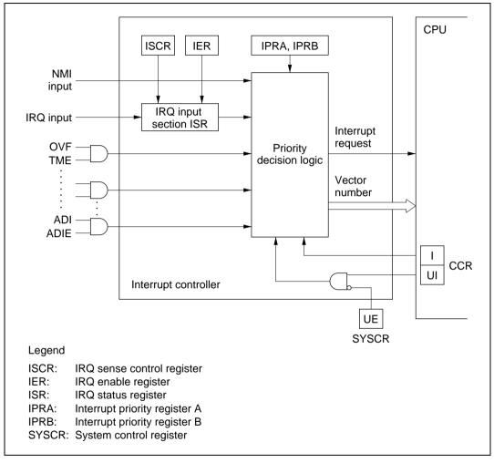
Figure 5.1 Interrupt Controller Block Diagram
