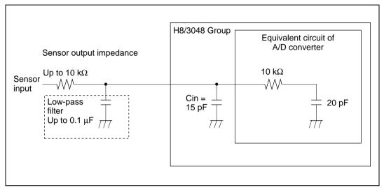
Figure 15.11 Analog Input Circuit (Example)
