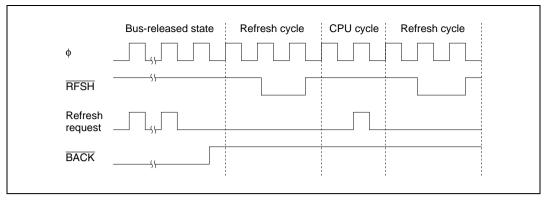
Figure 7.24 Refresh Cycles when Bus is Released
