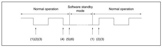
Figure 14.9 Procedure for Stopping and Restarting the Clock
