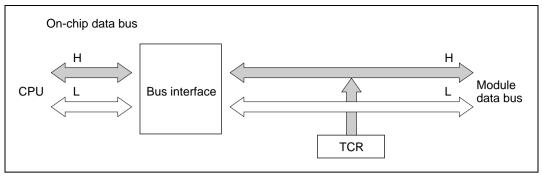
Figure 10.13 Access to Timer Counter (CPU Reads TCR)
