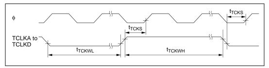
Figure 22.25 ITU External Clock Input Timing
