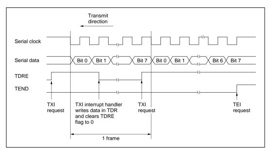
Figure 13.17 Example of SCI Transmit Operation
