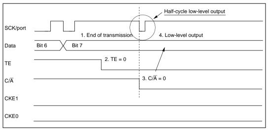
Figure 13.23 Operation when Switching from SCK Pin Function to Port Pin Function
