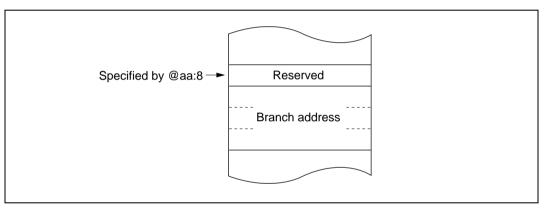
Figure 2.10 Memory-Indirect Branch Address Specification
