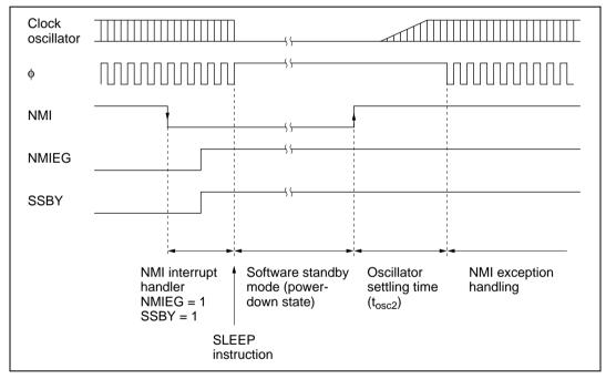
Figure 21.1 NMI Timing for Software Standby Mode (Example)
