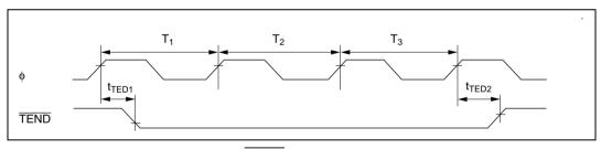
Figure 22.29 DMAC TEND Output Timing for 3 State Access
