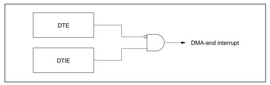
Figure 8.25 DMA-End Interrupt Logic
