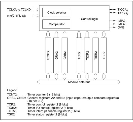
Figure 10.3 Block Diagram of Channel 2
