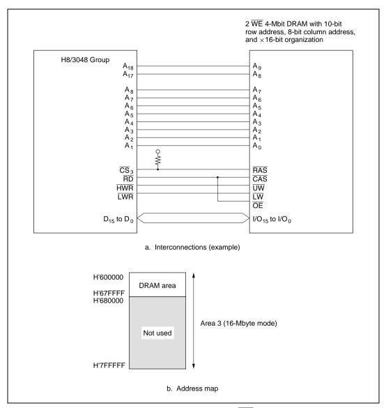
Figure 7.9 Interconnections and Address Map for 2WE 4-Mbit DRAM (Example)
