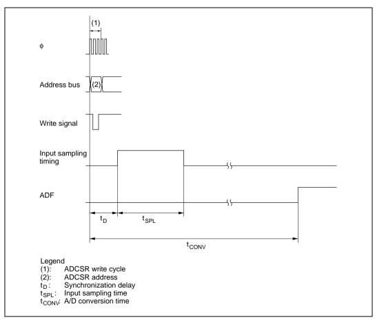
Figure 15.5 A/D Conversion Timing
