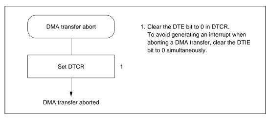
Figure 8.22 Procedure for Aborting a DMA Transfer
