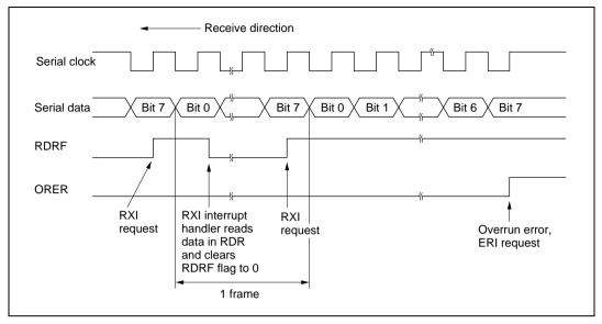
Figure 13.19 Example of SCI Receive Operation
