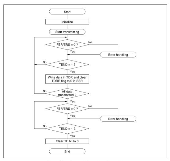
Figure 14.4 Transmit Flowchart (Example)
