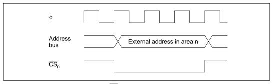
Figure 6.3  $\overline{CS}_n$  Output Timing (n = 7 to 0)
