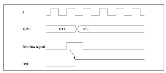
Figure 12.6 Timing of Setting of OVF
