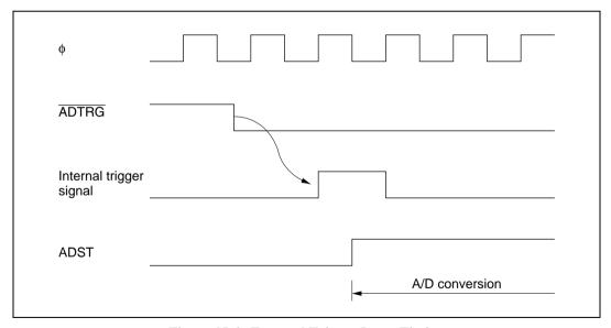
Figure 15.6 External Trigger Input Timing
