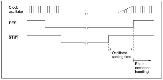
Figure 21.2 Hardware Standby Mode Timing
