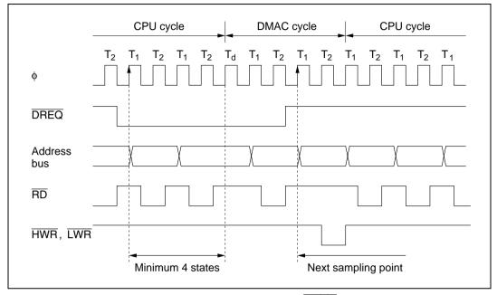
Figure 8.17 Timing of DMAC Activation by Low DREQ Level in Normal Mode
