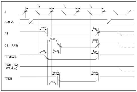
Figure 22.11 DRAM Bus Timing (Refresh Cycle): Three-State Access
