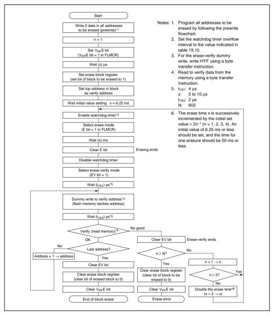
Figure 19.10 Erasing Flowchart
