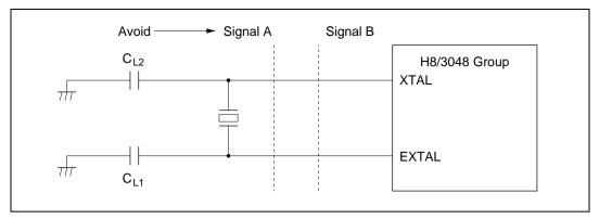
Figure 20.4 Example of Incorrect Board Design
