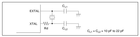
Figure 20.2 Connection of Crystal Resonator (Example)
