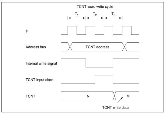
Figure 10.62 Contention between TCNT Word Write and Increment
