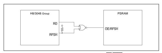
Figure 7.17 Interconnection to Pseudo-Static RAM with OE/RFSH Signal (Example)
