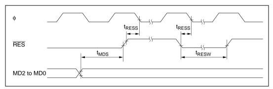
Figure 22.18 Reset Input Timing
