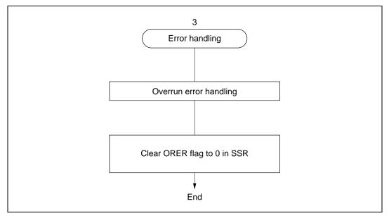
Figure 13.18 Sample Flowchart for Serial Receiving (2)
