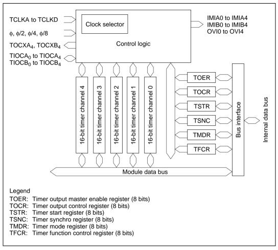
Figure 10.1 ITU Block Diagram (Overall)
