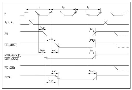
Figure 22.14 DRAM Bus Timing (Refresh Cycle): Three-State Access
