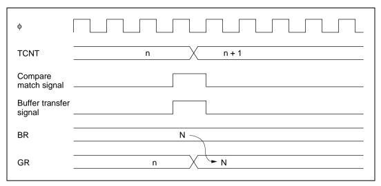
Figure 10.50 Compare Match and Buffer Transfer Timing (Example)
