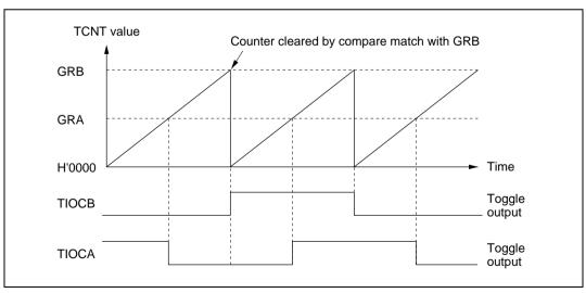
Figure 10.21 Toggle Output (Example)
