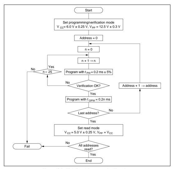
Figure 18.4 High-Speed Programming Flowchart
