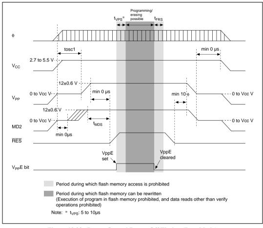
Figure 19.22 Power-On and Power-Off Timing (Boot Mode)
