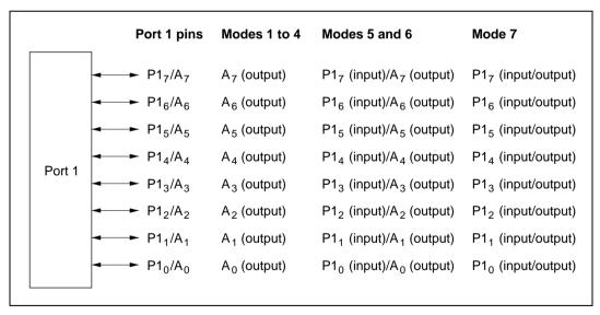
Figure 9.1 Port 1 Pin Configuration
