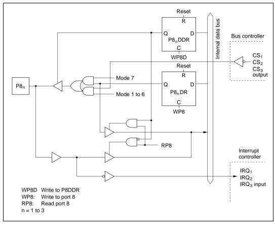
Figure C.8 (b) Port 8 Block Diagram (Pins P8<sub>1</sub> to P8<sub>3</sub>)
