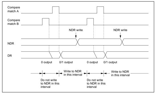
Figure 11.10 Non-Overlapping Operation and NDR Write Timing
