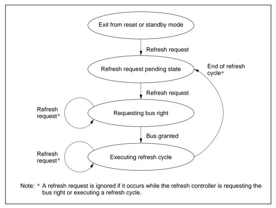
Figure 7.3 State Transitions for Refresh Cycle Execution
