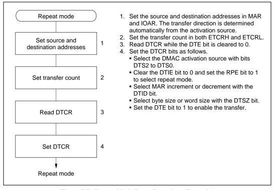
Figure 8.7 Repeat Mode Setup Procedure (Example)
