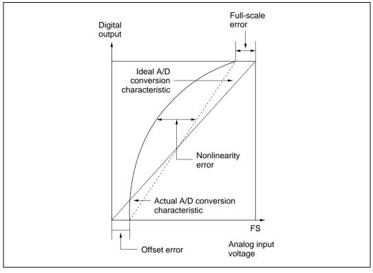
Figure 15.10 A/D Converter Accuracy Definitions (2)
