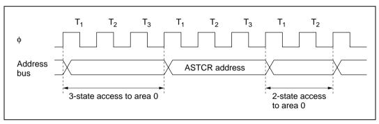
Figure 6.20 ASTCR Write Timing
