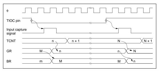
Figure 10.52 Input Capture and Buffer Transfer Timing (Example)
