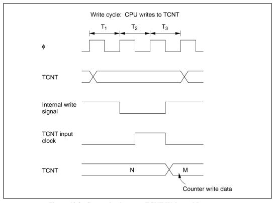
Figure 12.8 Contention between TCNT Write and Increment
