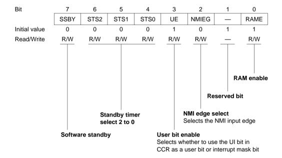
Bit 3—User Bit Enable (UE): Selects whether to use the UI bit in CCR as a user bit or an interrupt mask bit.
