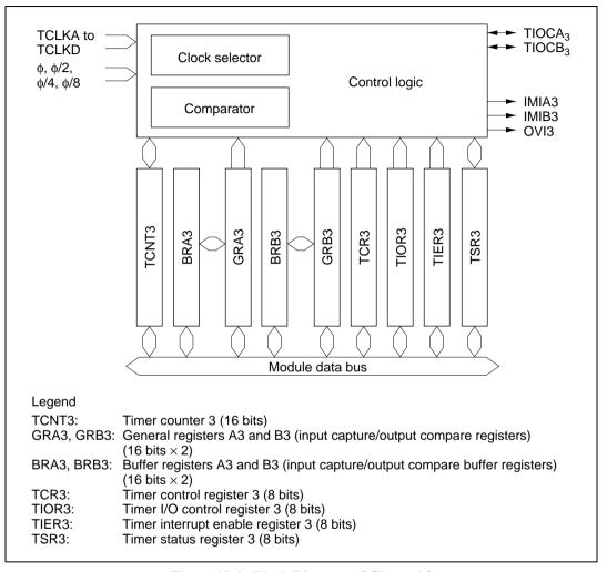
Figure 10.4 Block Diagram of Channel 3
