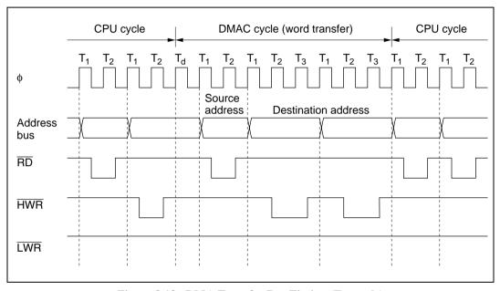
Figure 8.13 DMA Transfer Bus Timing (Example)
