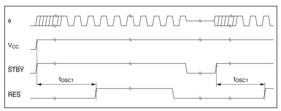
Figure 22.22 Oscillator Settling Timing
