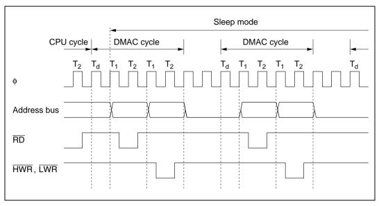
Figure 8.24 Timing of Cycle-Steal Transfer in Sleep Mode
