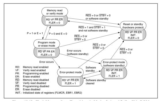
Figure 19.13 Flash Memory State Transitions in Modes 5, 6, and 7 (On-Chip ROM Enabled) when Programming Voltage (V<sub>PP</sub>) is Applied
