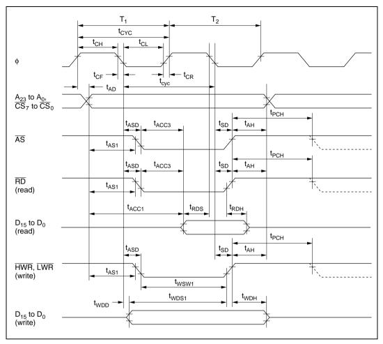
Figure 22.7 Basic Bus Cycle: Two-State Access
