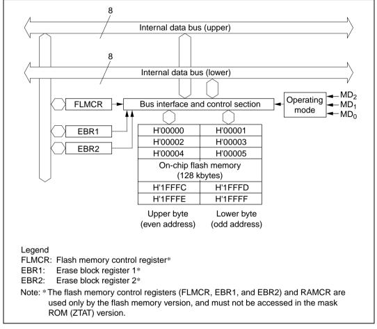
Figure 19.1 Flash Memory Block Diagram
