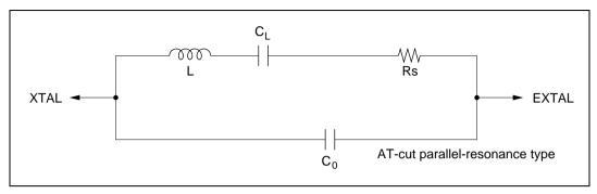
Figure 20.3 Crystal Resonator Equivalent Circuit
