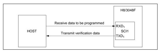
Figure 19.3 Boot-Mode System Configuration
