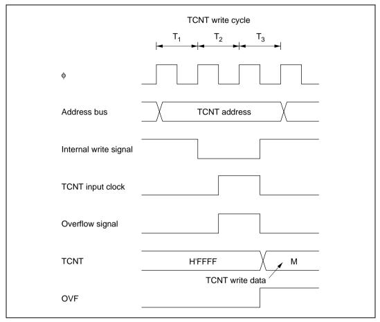
Figure 10.65 Contention between TCNT Write and Overflow
