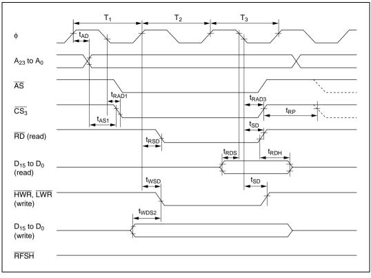
Figure 22.16 PSRAM Bus Timing (Read/Write): Three-State Access
