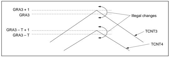
Figure 10.40 Changing a General Register Setting by Buffer Transfer (Caution 1)
