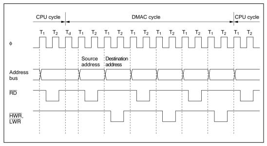
Figure 8.15 Bus Timing of Burst Mode DMA Transfer
