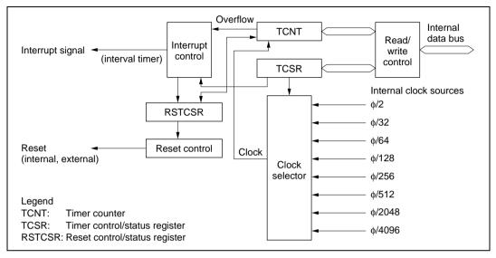
Figure 12.1 WDT Block Diagram
