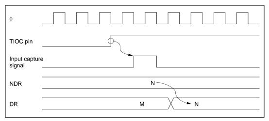
Figure 11.8 TPC Output Triggering by Input Capture (Example)
