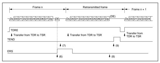
Figure 14.12 Retransmission in SCI Transmit Mode
