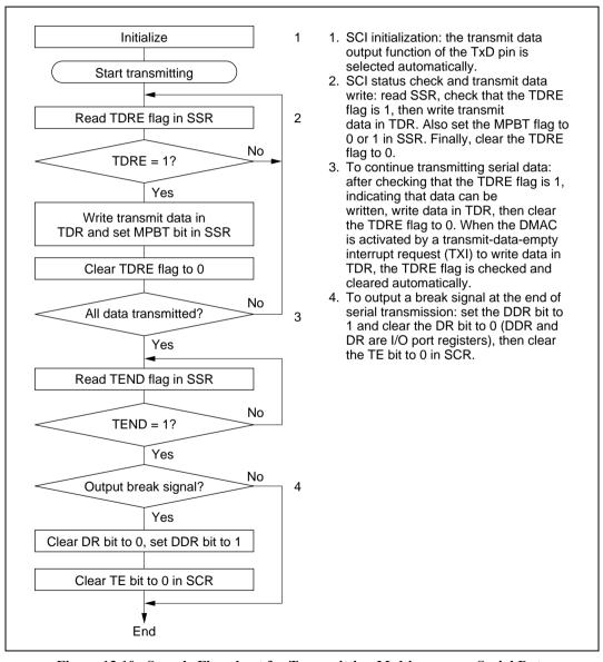
Figure 13.10 Sample Flowchart for Transmitting Multiprocessor Serial Data
