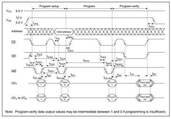
Figure 19.20 High-Speed, High-Reliability Programming Timing
