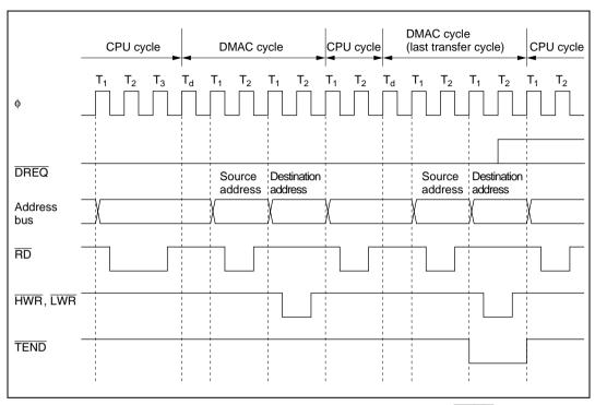
Figure 8.14 Bus Timing of DMA Transfer Requested by Low DREQ Input
