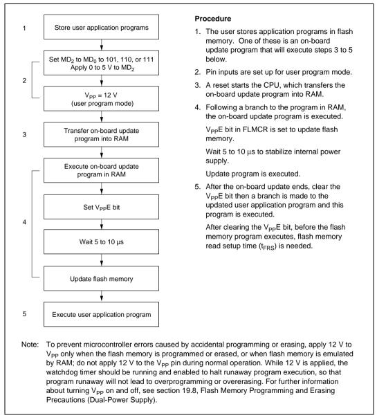
Figure 19.7 User Program Mode Operation (Example)
