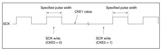
Figure 14.8 Clock Output Fixed Timing
