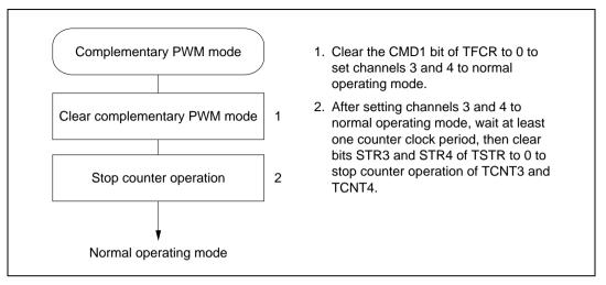
Figure 10.34 Clearing Procedure for Complementary PWM Mode
