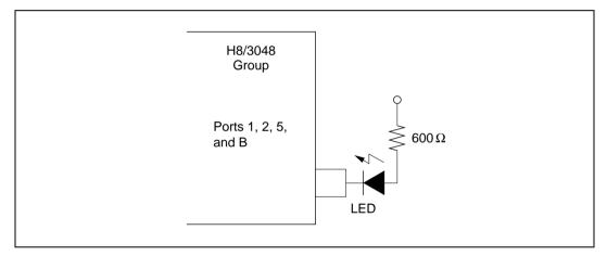
Figure 22.2 LED Drive Circuit (Example)
