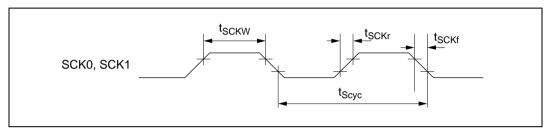
Figure 22.26 SCK Input Clock Timing
