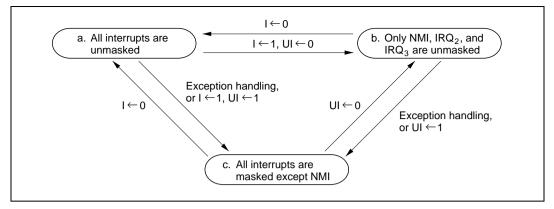
Figure 5.5 Interrupt Masking State Transitions (Example)
