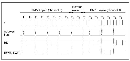
Figure 8.20 Bus Timing of Refresh Controller and DMAC
