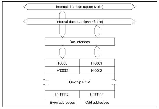
Figure 18.1 ROM Block Diagram (H8/3048, Mode 7)
