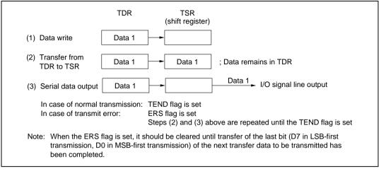
Figure 14.5 Relation Between Transmit Operation and Internal Registers
