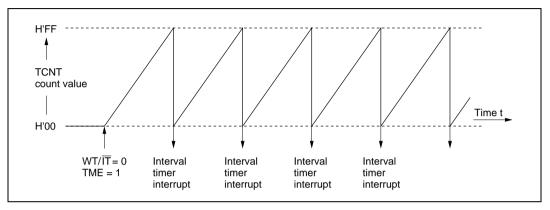
Figure 12.5 Interval Timer Operation
