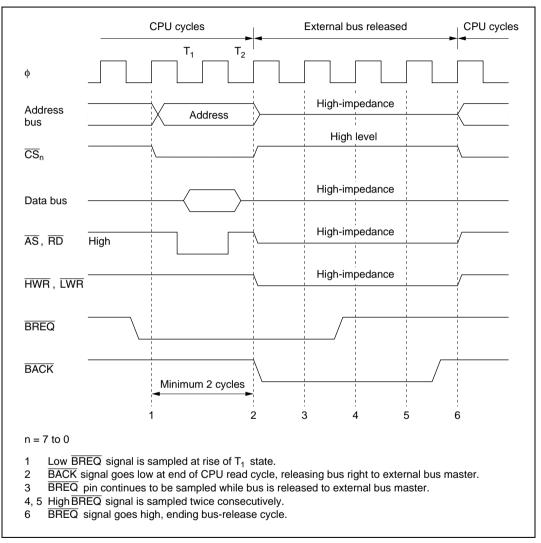
Figure 6.19 External-Bus-Released State (Two-State-Access Area, During Read Cycle)
