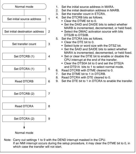
Figure 8.9 Normal Mode Setup Procedure (Example)
