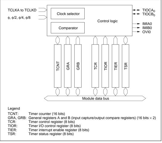
Figure 10.2 Block Diagram of Channels 0 and 1 (for Channel 0)
