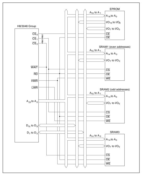
Figure 6.18 Interconnections with Memory (Example)
