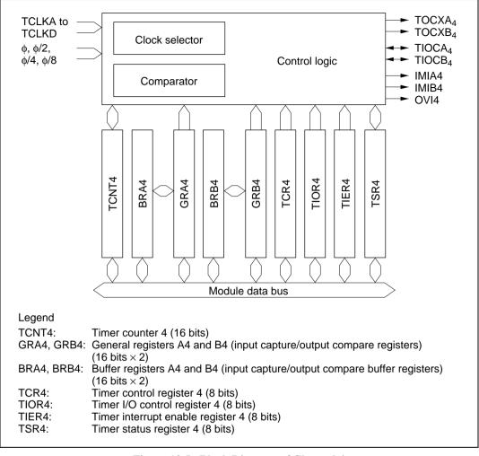
Figure 10.5 Block Diagram of Channel 4
