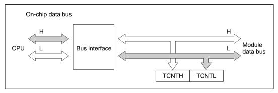
Figure 10.9 Access to Timer Counter (CPU Writes to TCNT, Lower Byte)
