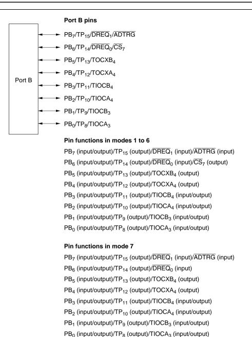
Figure 9.11 Port B Pin Configuration
