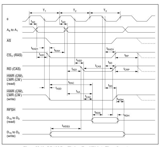
Figure 22.10 DRAM Bus Timing (Read/Write): Three-State Access
