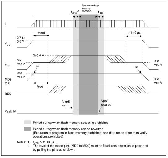
Figure 19.23 Power-On and Power-Off Timing (User Program Mode)
