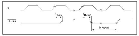
Figure 22.19 Reset Output Timing\*
