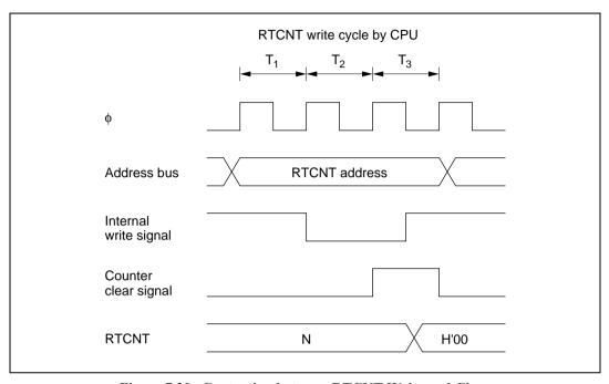
Figure 7.20 Contention between RTCNT Write and Clear
