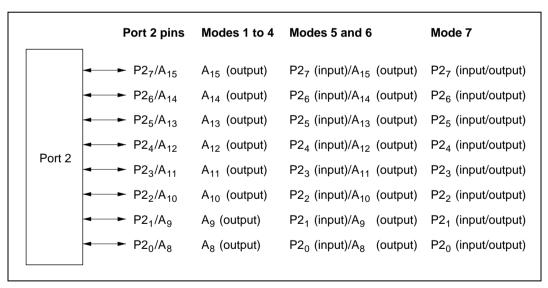
Figure 9.2 Port 2 Pin Configuration
