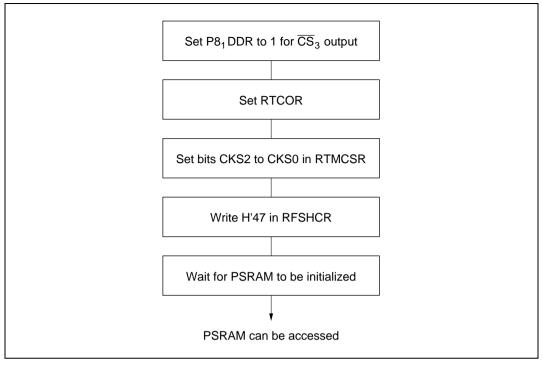
Figure 7.18 Setup Procedure for Pseudo-Static RAM
