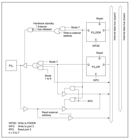
Figure C.3 Port 3 Block Diagram
