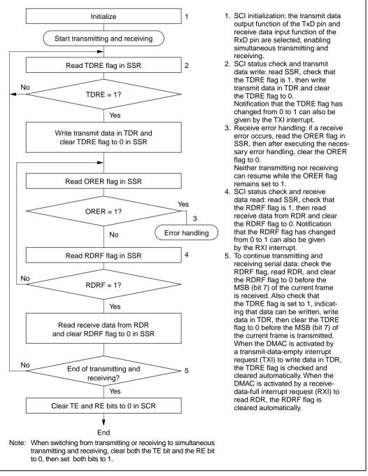
Figure 13.20 Sample Flowchart for Serial Transmitting
