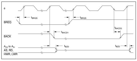
Figure 22.21 Bus-Release Mode Timing
