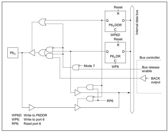
Figure C.6 (c) Port 6 Block Diagram (Pin P62)
