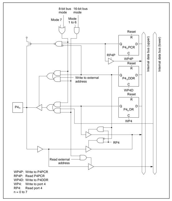
Figure C.4 Port 4 Block Diagram
