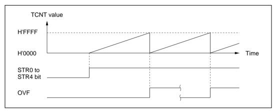
Figure 10.15 Free-Running Counter Operation
