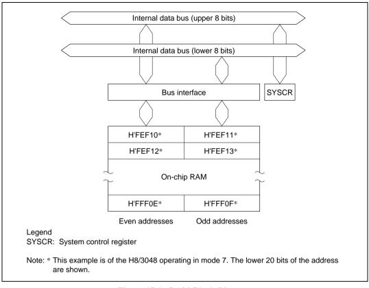
Figure 17.1 RAM Block Diagram
