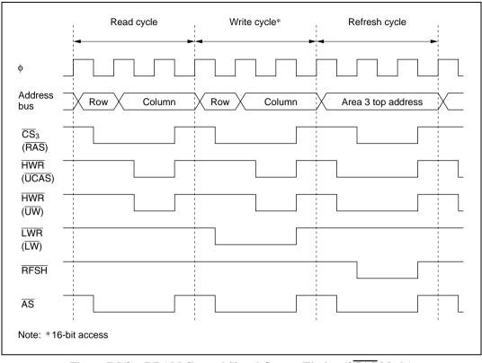
Figure 7.5(2) DRAM Control Signal Output Timing (2CAS Mode)
