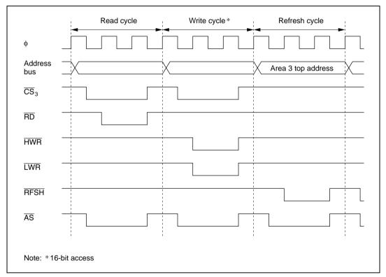
Figure 7.15 Pseudo-Static RAM Control Signal Output Timing
