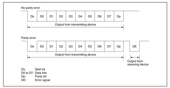
Figure 14.3 Smart Card Interface Data Format
