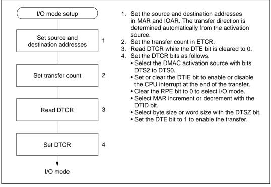
Figure 8.3 I/O Mode Setup Procedure (Example)
