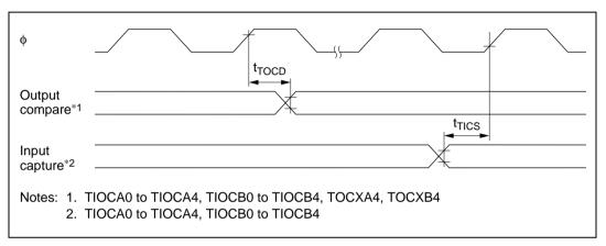
Figure 22.24 ITU Input/Output Timing
