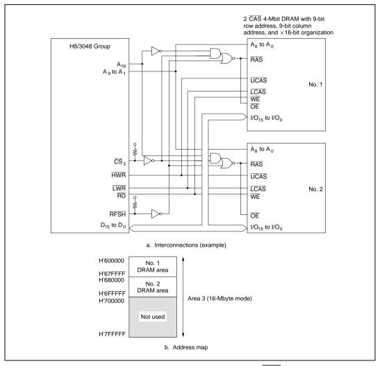
Figure 7.13 Interconnections and Address Map for Multiple 2CAS 4-Mbit DRAM Chips (Example)
