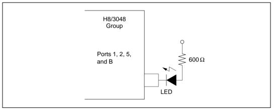
Figure 22.5 LED Drive Circuit (Example)
