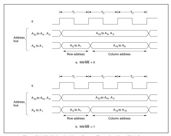
Figure 7.4 Multiplexed Address Output (Example without Wait States)
