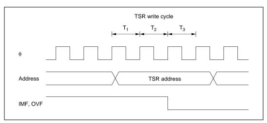
Figure 10.60 Timing of Clearing of Status Flags
