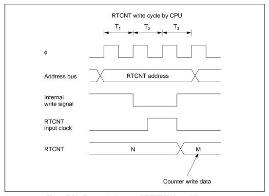
Figure 7.21 Contention between RTCNT Write and Increment
