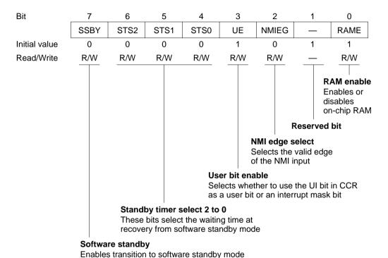
**Bit 7—Software Standby (SSBY):** Enables transition to software standby mode. (For further information about software standby mode see section 21, Power-Down State.)
