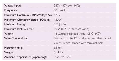
In order to protect the surrounding environment, this surge protection device must be enclosed in a luminaire that can contain flames and sparks, which may occur in case of malfunction, such as overvoltage power connection (ex:600V).
