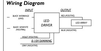
Input, output and 0-10V Dimming use lead-wires. Lead-wires are 18AWG 105C/600V solid copper.
