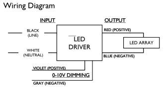
Input, Output and 0-10V Dimming use lead-wires. Lead-wires are 18AWG 105C/600V solid copper
