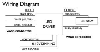
Input is Wago 3-position wire trap connector – use 18AWG solid or tinned stranded.
