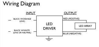
Input and Output: 18AWG 105C/600V solid copper lead wires
