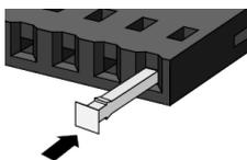
Polarization keys (keys to plug into the housings to ensure polarization)
