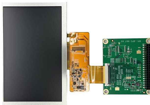
Figure 14. FPC connection between 5-inch Tianma LCD panel and adapter board
