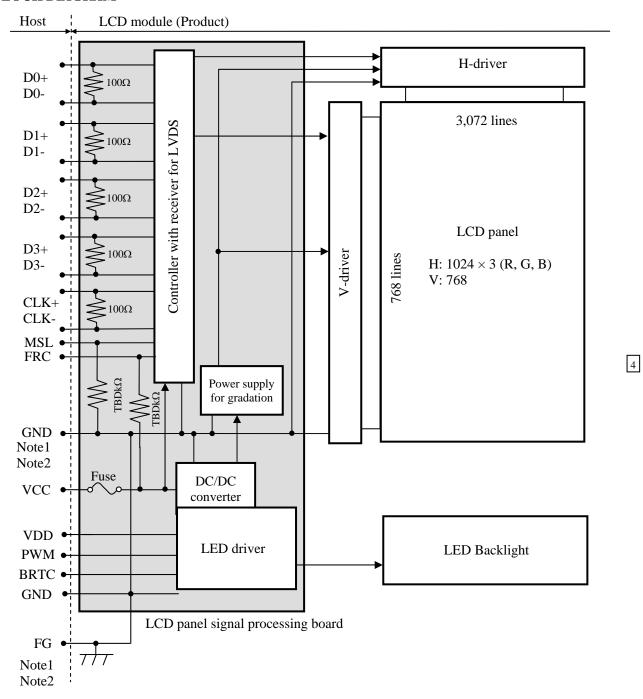
Note1: Relations between GND (Signal ground and LED driver ground) and FG (Frame ground) in the LCD module are as follows.
