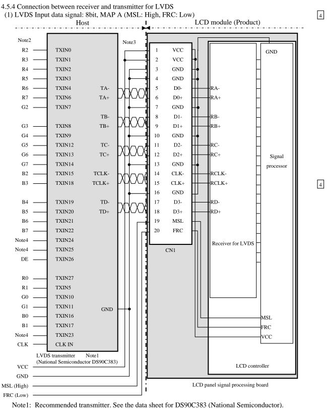
Note2: LSB (Least Significant Bit) - R0, G0, B0 MSB (Most Significant Bit) - R7, G7, B7
