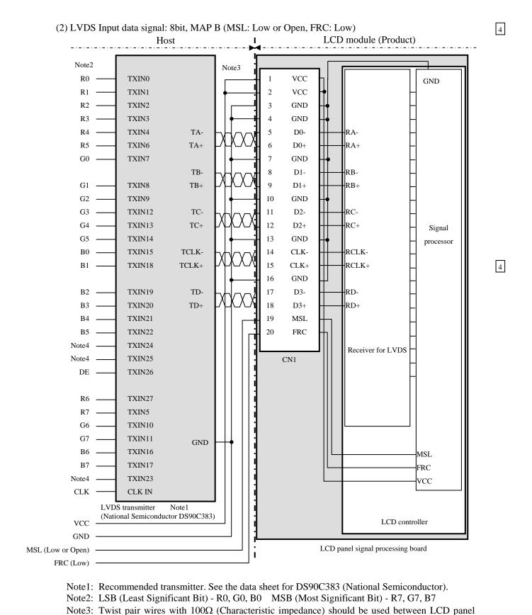
Note4: Input signals to TXIN23, TXIN24 and TXIN25 are not used inside the product, but do not
