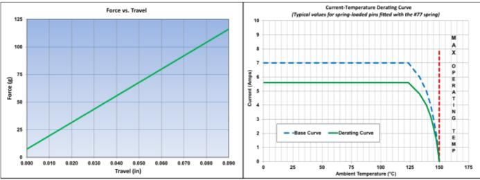
The stroke, force and current rating values are measured using spring pins with an internal construction per the design specification. Individual spring pin performance may vary from these values based on design differences.
