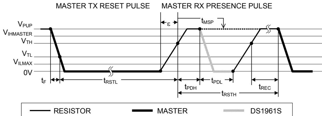
After the bus master has released the line it goes into receive mode (RX). Now the 1-Wire bus is pulled to  $V_{PUP}$  through the pullup resistor or, in case of a DS2480B driver, by active circuitry. When the threshold  $V_{TH}$  is crossed, the DS1961S waits for  $t_{PDH}$  and then transmits a presence pulse by pulling the line low for  $t_{PDL}$ . To detect a presence pulse, the master must test the logical state of the 1-Wire line at  $t_{MSP}$ .
