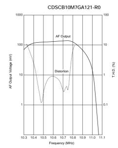
$\begin{array}{l} Input = 100 dB\mu \\ fdev. = \pm 75 kHz \\ fmod. = 1 kHz \\ Vcc = 3.2 V \end{array}$
