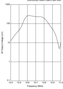
$\begin{array}{ll} \text{Input} &= 100 \text{dB} \mu \\ \text{fdev.} &= \pm 50 \text{kHz} \\ \text{fmod.} &= 1 \text{kHz} \\ \text{Vcc} &= 5.0 \text{V} \end{array}$
