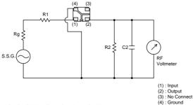
R1+Rg=R2=Input/Output Impedance, Rg=50Ω
