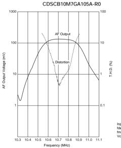
$\begin{array}{ll} \text{Input} &= 100 \text{dB} \mu \\ \text{fdev.} &= \pm 75 \text{kHz} \\ \text{fmod.} &= 1 \text{kHz} \\ \text{Vcc.} &= 3.0 \text{V} \end{array}$
