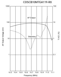
$\begin{array}{l} Input = 100 dB \mu \\ fdev. = \pm 60 kHz \\ fmod. = 1 kHz \\ Vcc = 3.0 V \end{array}$
