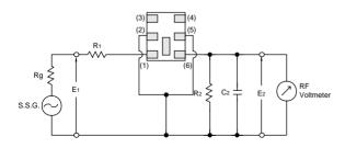
$\begin{array}{cccc} Rg = 50\Omega & R1 = 280\Omega \pm 5\% & R2 = 330\Omega \pm 5\% \\ C_2 = 10 \pm 2 & pF & (Including stray capacitance an of RF Volt Meter) \\ E_1: S.S.G. & Output Voltage \end{array}$
