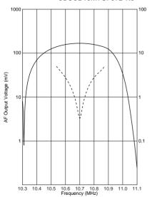
$\begin{aligned} & \text{Input} = 100 \text{dB}\mu \\ & \text{fdev.} = \pm 80 \text{kHz} \\ & \text{fmod.} = 1 \text{kHz} \\ & \text{Vcc} = 3.0 \text{V} \end{aligned}$
