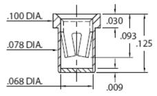
9873-0-XX-XX-02-XX-10-0 Solder mount in Ø.083±.003 PTH. #02 Contact for Ø.040-.050 pins. Also available on 12mm wide carrier tape: 4,500 parts per 13" reel.
