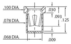
9873-0-XX-XX-02-XX-10-0 Solder mount in Ø.083±.003 PTH. #02 Contact for Ø.040-.050 pins. Also available on 12mm wide carrier tape: 4,500 parts per 13" reel.
