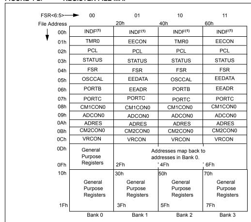
Note 1: Not a physical register. See Section 4.8 "Indirect Data Addressing: INDF and FSR Registers".
