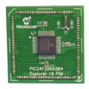
This 100-pin Plug-in Module comes fitted with a PIC24F32KA304 device in a 44-pin TQFP package. Use it as a plug-in module with the Explorer 16 board (DM240001) for development of your extreme low-power, touch-sense or general purpose control applications.
