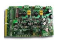
Buck/Boost Converter PICtail™ Plus Daughter Board provides an easy and economical development platform for dsPIC® SMPS and Digital Power Conversion GS family Digital Signal Controllers which are designed to provide low-cost and efficient control for wide range of power supply topologies and power conversion applications.
