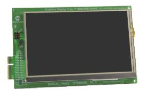
The Graphics Display Truly 7" 800x480 Board is a demonstration board for evaluating Microchip's graphic display solution and graphics library for 16- and 32-bit microcontrollers. It is an expansion board compatible with the Graphics LCD Controller PICtail™ Plus S1D13517 Board (AC164127-7).
