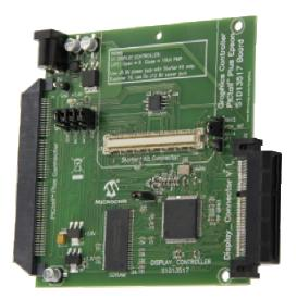
The Graphics Controller PICtail<sup>™</sup> Plus Epson S1D13517 Board allows evaluating Microchip Technology's solution and graphics library for 16and 32-bit microcontrollers. The Epson S1D13517 offers hardware acceleration for alpha-blending, transparency, animation, multiple buffering, and picture in picture. The kit is compatible with the Explorer 16 development board (DM240001) or one of the PIC32 Starter Boards (DM320001, DM320003).
