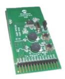
The rfPIC 433 Mhz transmitter works with the receiver attached to the PICkit(tm) 1 Flash Starter Kit. It is a component of the rfPIC Development Kit (DV164102).
