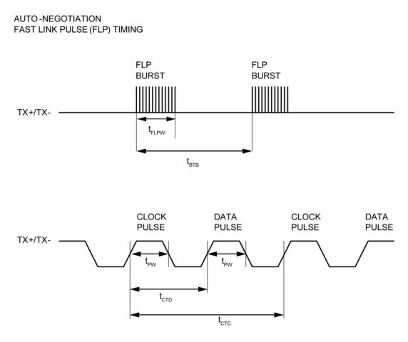
Figure 12. Auto-Negotiation Fast Link Pulse (FLP) Timing
