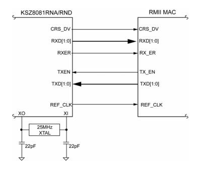
Figure 2. KSZ8081RNA/RND RMII Interface (RMII - 25MHz Clock Mode)
