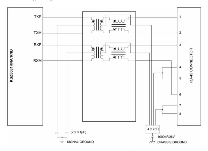
Figure 20. Typical Magnetic Interface Circuit
