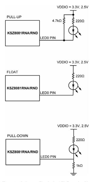
Figure 17. Reference Circuits for LED Strapping Pins
