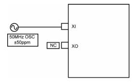
Figure 19. 50MHz Oscillator Reference Clock Connection
