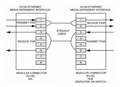
Figure 5. Typical Straight Cable Connection
