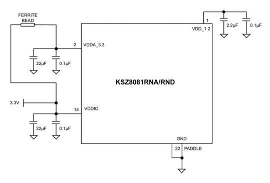
Figure 9. KSZ8081RNA/RND Power and Ground Connections
