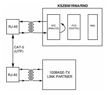
Figure 8. Remote (Analog) Loopback
