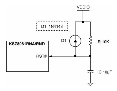
Figure 15. Recommended Reset Circuit
