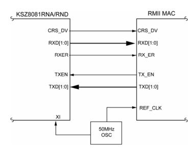
Figure 3. KSZ8081RNA/RND RMII Interface (RMII – 50MHz Clock Mode)
