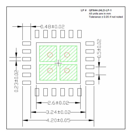
Figure 21. Recommended Land Pattern, 24-Pin (4mm x 4mm) QFN
