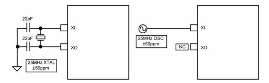
Figure 18. 25MHz Crystal/Oscillator Reference Clock Connection
