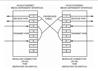
Figure 6. Typical Crossover Cable Connection
