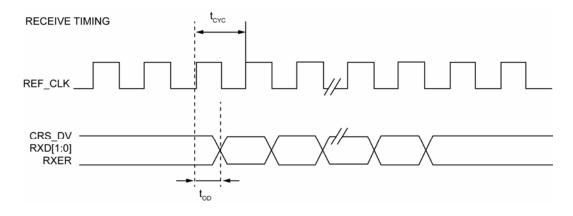
Figure 11. RMII Timing - Data Input to RMII
