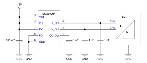
$<sup>^{</sup>st}$  if the supply voltage is disturbed by EMI it can be useful to place a second capacitor (100 pF ceramic) parallel to the 100nF capacitor.
