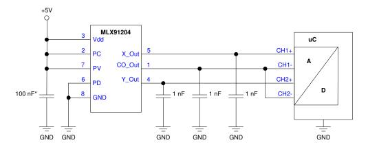
$<sup>^{</sup>st}$  if the supply voltage is disturbed by EMI it can be useful to place a second capacitor (100pF ceramic) parallel to the 100 nF capacitor.
