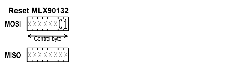
Figure 9: SPI communication reset the MLX90132
