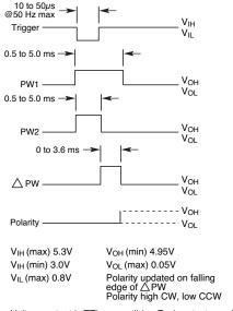
Voltage output is TTL compatible. Each output can drive one low power Schottky or multiple CMOS devices.
