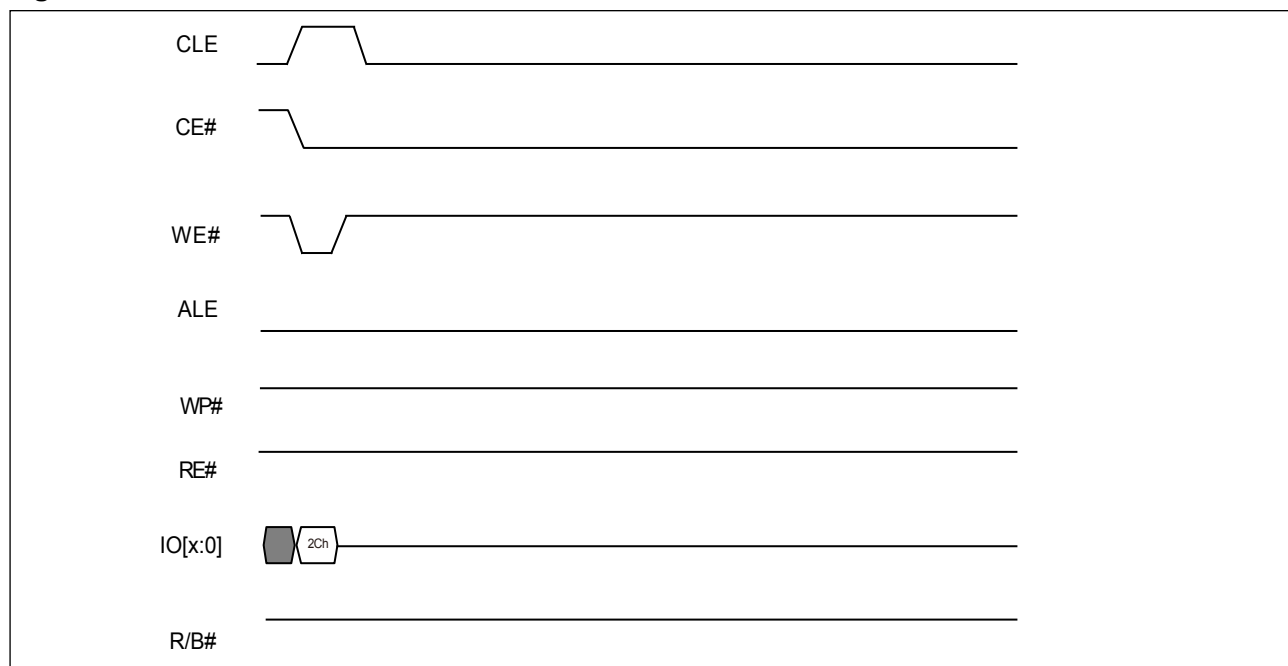
Figure 39. AC Waveforms for Block Solid-Protect
