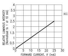
Fig3. Relative Luminous Intensity vs. DC Forward Current
