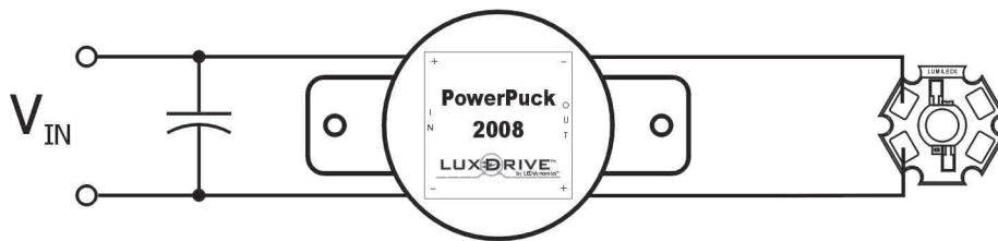
Figure 17. Place a capacitor across the input terminals when the distance to the DC power source is greater than 18 inches
