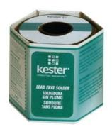
331 Organic flux is a water soluble formula for use in flux-cored solder wire and is more effective than rosin fluxes in solder difficult metal. The flux is more heat stable than most organic fluxes, resulting in minimal smoke and order. The residue can be completely removed with a simple water rinse.
