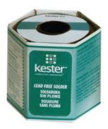
331 is designed for optimal cleanability with water. Highly active water-soluble flux for solerding difficult metals. Classified as ORH1 per J-STD-004. All organic water soluble core solder are 3% flux.
