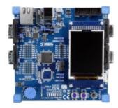
The Keil MCB1750 Evaluation Board introduces the new NXP LPC1750 family of ARM Cortex-M3 processor-based devices, allowing you to create and test working programs for this advanced architecture. The MCB1750 has a wide range of interfaces making it a great starting point for your next Cortex-M3 project.
