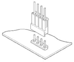
The directional features of the housing preveinsertion.
