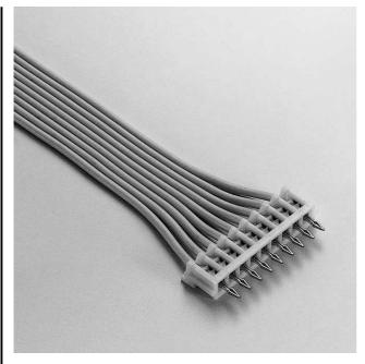
This is a 2.5mm (.098") pitch insulation displacement connector that is soldered directly onto printed circuit boards, with a mounting height of 7.1mm (.280") and with a width of 4.1mm (.161"). The DB connectors can be used by themselves or in combination with NR or HR connectors.
