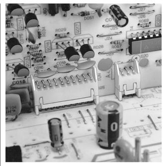
This 2.5mm (.098") pitch connector is used to interconnect printed circuit boards. It easily resists distortion during mating, thus ensuring reliable contact, even under adverse conditions.
