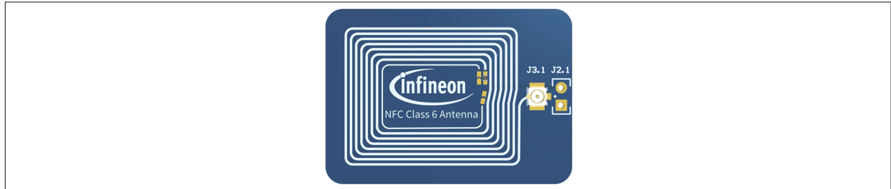
Figure 9 Class 6 shield antenna in its default configuration (usage with the included UMCC cable)
