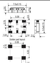
Pad Connections 1. Voltage Control 2. GND 3. Output 4. +Vs T1, T2, T3, T4, Do Not Connect
