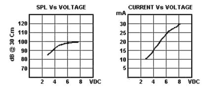
\*\*Note - Frequency is 2.8 KHz. + 0.2 KHz. from 3 to 8 VDC
