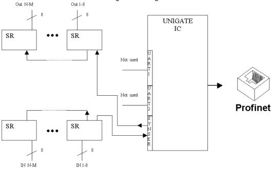
Version 2: Use of UNIGATE® IC for digital or analog I/O-modules
