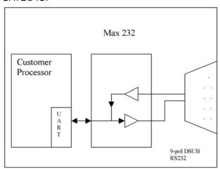
Your device, which on the whole is supposed to be assembled as shown above, will now be modified in a way that the Profinet is available at the 9-pol. socket. However, a hardware redesign is necessary in order to keep the assignment in standard form.
