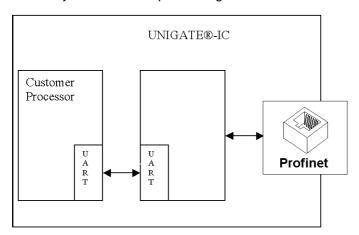
After the RS232-driver has been replaced by the UNIGATE® IC, Profinet is available at an RJ45-socket.
