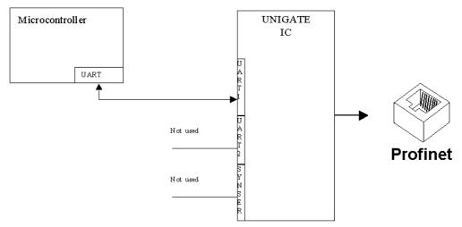
The UNIGATE® IC independently processes the communication with the customer's device via the TTL-interface.
