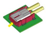
(2) Continue to rotate it upwards and release the rear lock portion.
