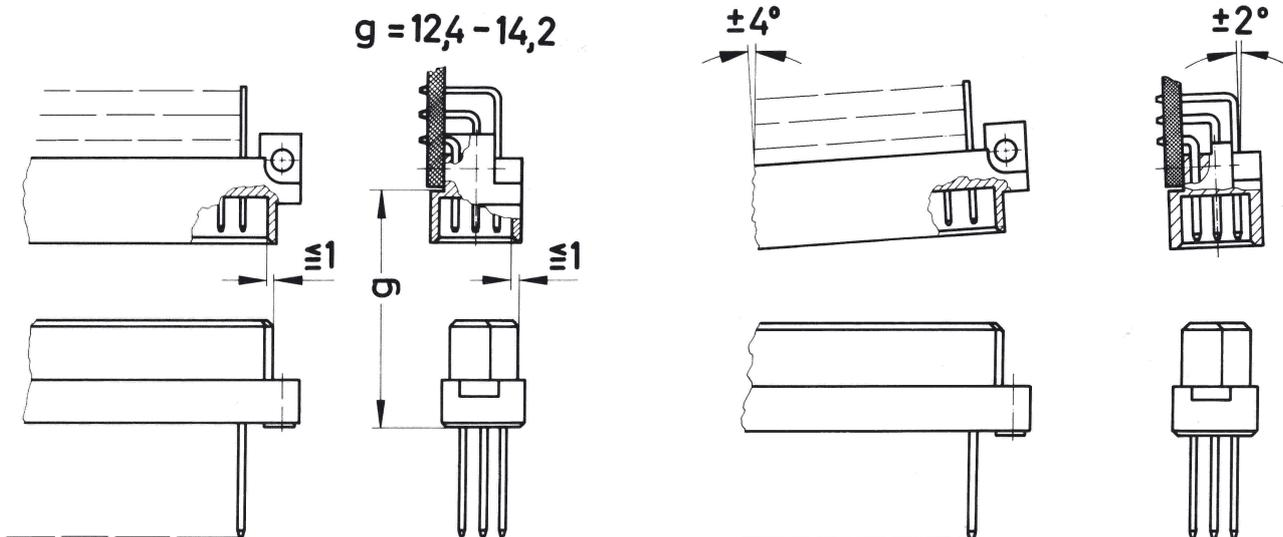
To ensure reliable connections and prevent unnecessary damage, please refer to the application data diagrams. These recommendations are set out in IEC 60603-2. The connectors should not be coupled and decoupled under electrical load.
