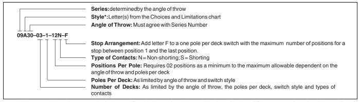
\* All rotary switches that are required to have military designated markings and testing adhering to MIL-3786 are to be ordered by specifying the military part number identified on the appropriate slash sheet. Specifications are subject to change. Please refer to the current datasheet on www.grayhill.com for the most current published specifications for this product.
