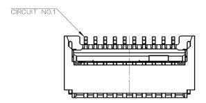
BM-Lite FFC connector. Pin 1 is to the left.
