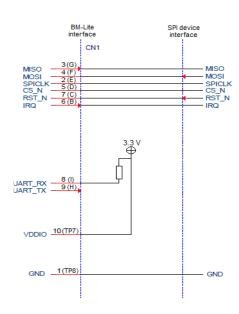
Example schematic of BM-Lite interface using SPI
