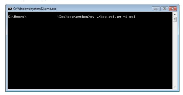
The script will now search through your COM ports and connect to the correct one. When the BEP host interface script starts, note that it states which COM port and baud rate it's using. These and other properties can be changed when running the script using the appropriate arguments as listed in the BM-Lite integration document.
