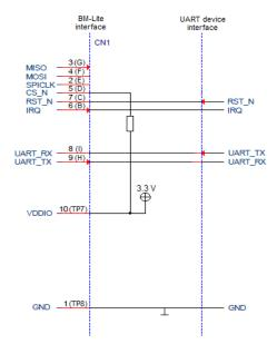
Schematic of BM-Lite interface using UART
