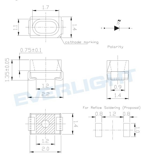
**Note**: Tolerance unless mentioned is  $\pm 0.1$ mm; Unit = mm
