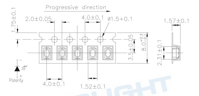
**Note**: Tolerance unless mentioned is  $\pm 0.1$ mm; Unit = mm
