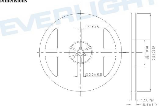
**Note**: Tolerance unless mentioned is  $\pm 0.1$ mm; Unit = mm
