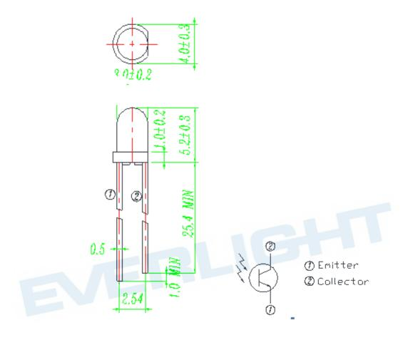
Note: Tolerances unless dimensions ±0.25mm
