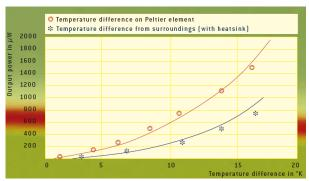
Output power from ECT 310 in combination with Peltier element TEC2L-15-15-15-5.6:
