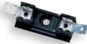
**S-8202** – Fuseblocks with 1/4" quick-connect terminals 300 volt rating. Available in 1 through 12 position units. Break-away design lets you snap off or combine positions as needed to get the exact number required for your application. UL recognized, 20 Amp max.
