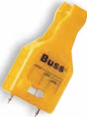
The **FT-3** combination fuse tester and fuse puller is designed for easy one-handed use. It tests glass and blade fuses in or out of the fuseblock. This continuity tester is for fuses in circuits up to 24V maximum. Light glows when fuse is good.
