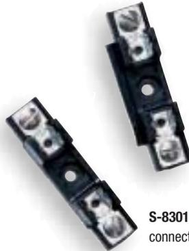
**S-8301** – Fuseblocks with screw connect terminals 300 volt rating. Available in 1 through 12 position units. Break-away design lets you snap off or combine positions as needed to get the exact number required for your application. UL recognized, 30 Amp max.
