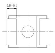
For reflow soldering (propose)
