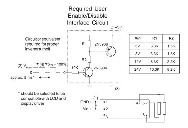
(1) Low ESR type input by-pass capacitor (22 uF - 100 uF) may be required to reduce reflected ripple.
