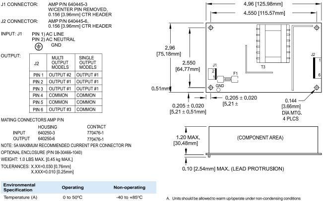
before application of power. Derate output current and total output power by 2.5% per °C above 50°C. В
